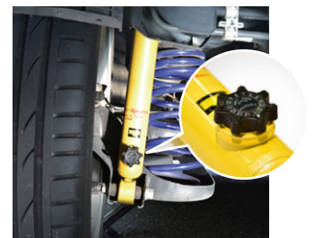
Lower Sports PLUS Suspension Kit system.
