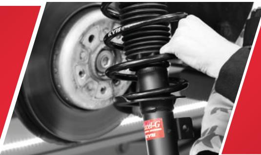
Occasionally, a shock absorber will be diagnosed as faulty when removed from its packaging for installation. However, this may not be the case and the fix is often very simple: priming.
