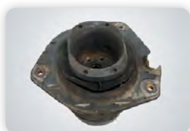
Torn Strut Insulator
