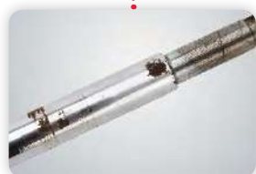
Damaged piston rod
